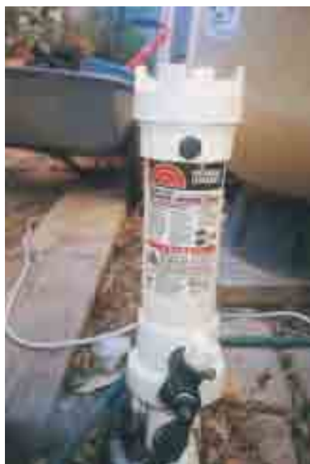
Figure 17 Erosion canister (erosion feeder)
