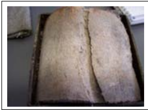
Figure 5(a) Splitting of specimen
