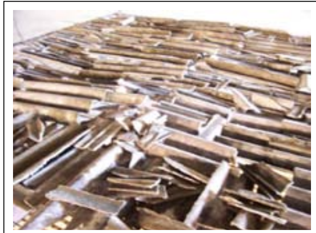
Figure 8 A/C sheeting placed on test frame
