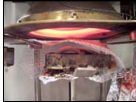
Test 3, Specimen #3 (shearing of A/C)
