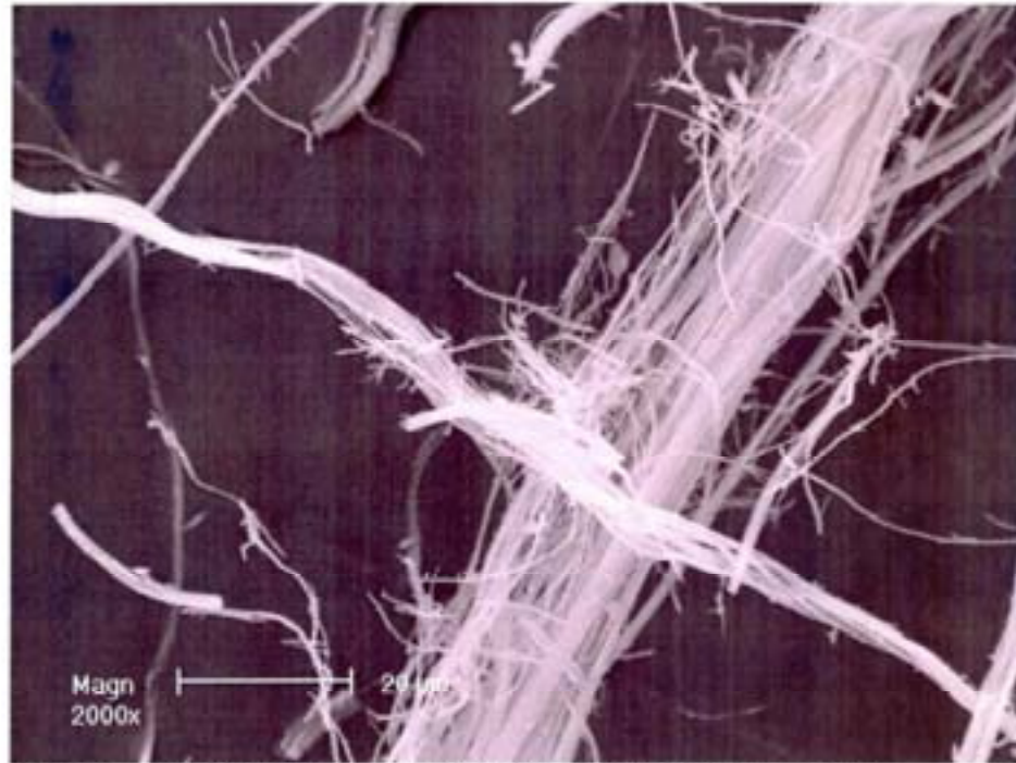
Reference sample of heat affected chrysotile (approx. 800 °C). EDAX spectrum shown.
