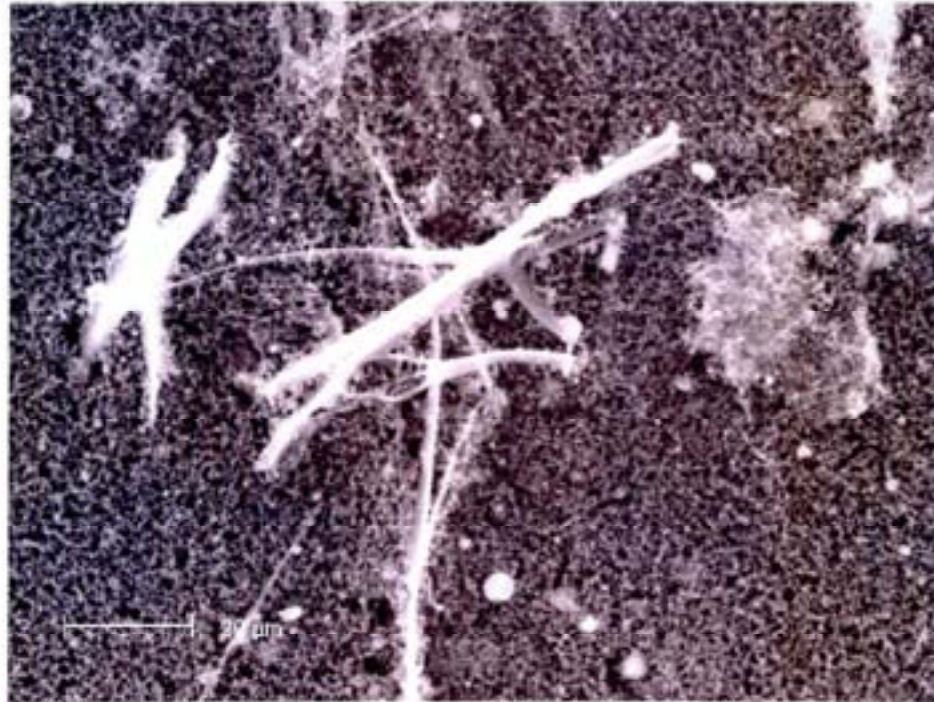
Filter No. A48, Fibre bundle with no crystalline structure, EDAX spectrum shown
