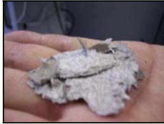
Test 1, Specimen #2 (exposed fibre after test)
