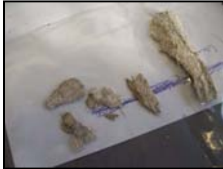
Test 3, Specimen #3 (spalled debris)
