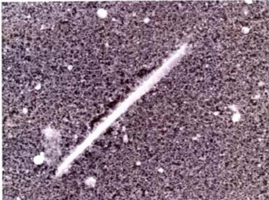
Filter No. A38, Fibre found with no crystalline structure, approximately 18 \mu\text{m} in length and 6 \mu\text{m} in diameter. EDAX spectrum shown
