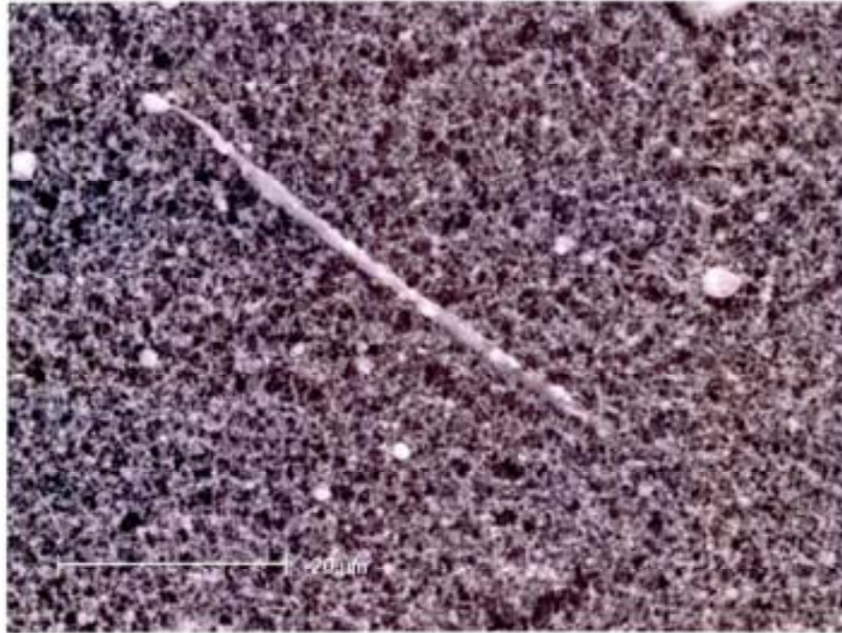
Filter No. A48, Fibre found with no crystal structure, EDAX spectrum shown
